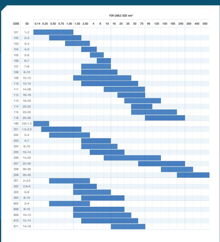
All the above data has an approximate value and refers exclusively to the diameters of single-cores. The appreciable differences in outside diameters of similar cable sections, are the result of differences in the thickness of the insulation of the cables. When choosing a sleeve according to cable section, please also refer to specific cable manufacturers data.
